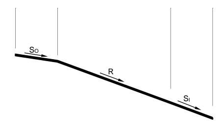
$S_0$  = Outside Shoulder Slope  $S_1$  = Inside Shoulder Slope R = Roadway Superelevation Rate
